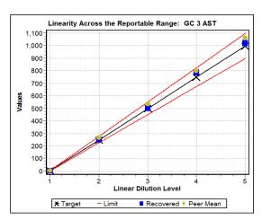
**Summary:** Maine Standards Company Technical Support advised that recovery and reproducibility was not consistent with Peers. In this case, a cracked syringe case caused the impression seen between repetitions. This case study emphasizes that calibration and running QC may not always detect instrument issues.
